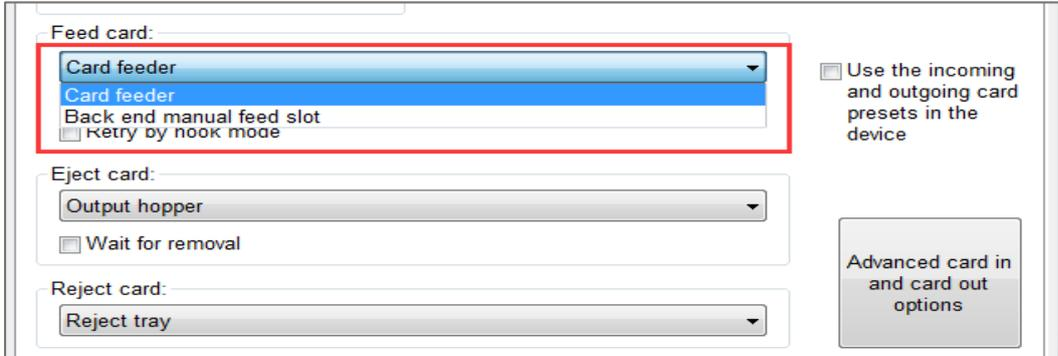
(2) Manual feeding card piece by piece from back end manual feed slot is optional.
