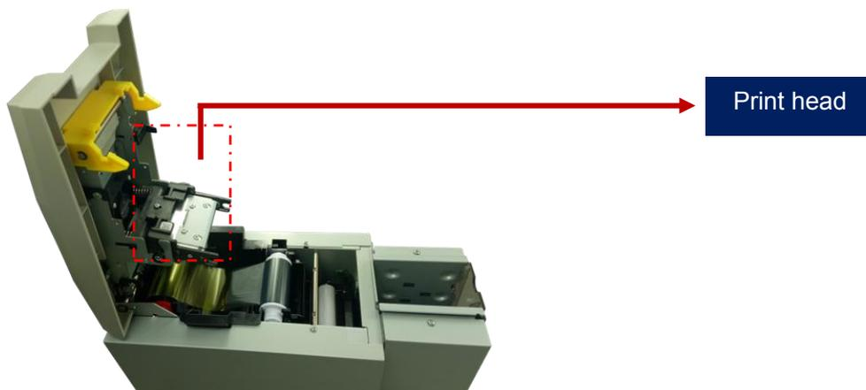
Step 3: Wipe the print head in one direction, from left to right or right to left with cleaning stick. Do not wipe back and forth. Generally wipe 3-5 times will be ok.
