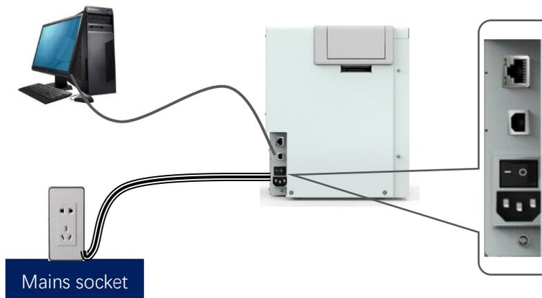
Ethernet communication interface installation: RJ45 network interface ,568B connection mode.
